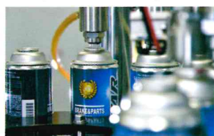
原液充填・ガス充填 Filling with undiluted solution & filling with gas
