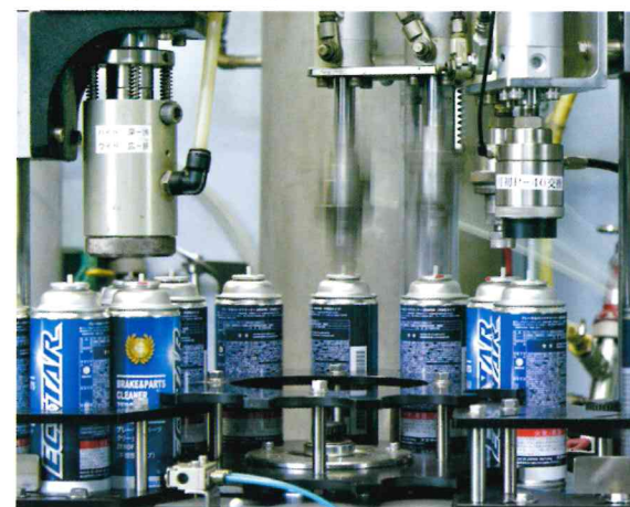
重量検査後、付属品等装着 Following weight inspection, installation of attachments, etc.
