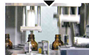
完全ドライ状態で液体充填 Filling of liquid in a completely dry state
